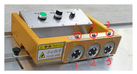
Circuit boards along the guide into the machine inside, can clean are separately blade and points in the process of plate stress to A minimum, depending on A, B, C three groups on the knife and the knife spacing is appropriate. So should be based on partitioned PCB thickness and material, to adjust the blade spacing. In order to achieve the best results. The basic principle of adjustment are as follows:
